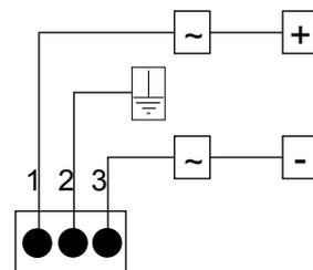
Earth connection - Although a terminal is offered for earth connection, the connection is optional. The instrument does not need this connection for correct functioning nor for compliance with the security regulations.
