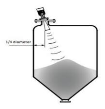
**Note:** During installation it is important to remember that in the proximity of the probe there is a BLIND ZONE (or BLIND DISTANCE) of 0.25 m which the sensor can not measure. (Figure D).
