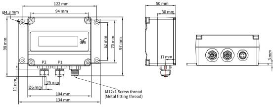
$\frak{P1/P2}$  : Connected to Ø6 PVC / PTFE compressed air pipe
