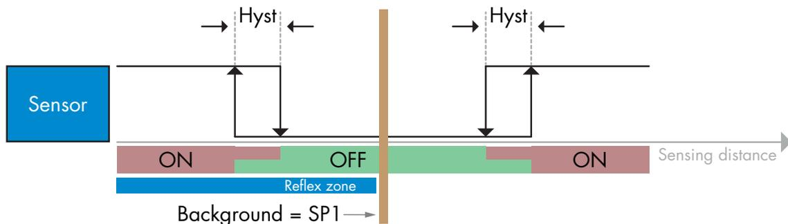
Example of presence detection - with non-inverted logic
