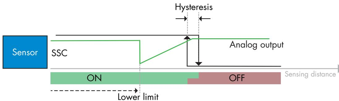
The two buttons for the single value auto-teach command are found in the "Parameters" menu. The following procedure defines the placement of the output slope. Please note, that the LEDs will flash to indicate IO-Link connection throughout the procedure.
