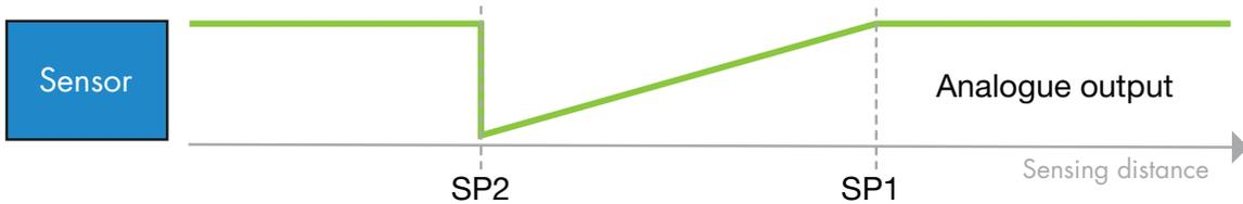
On the other hand, if SP2 is located closer to the sensor than SP1, then the result is a falling slope.
