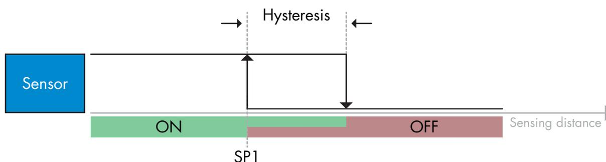
This teach-procedure affects the output of Pin4, and it saves one value for setpoint 1 (SP1). The button is found in the Parameters menu: 'Setpoint 1 Single Value Teach'. Prepare the installation by mounting the sensor and preparing the target placement.
