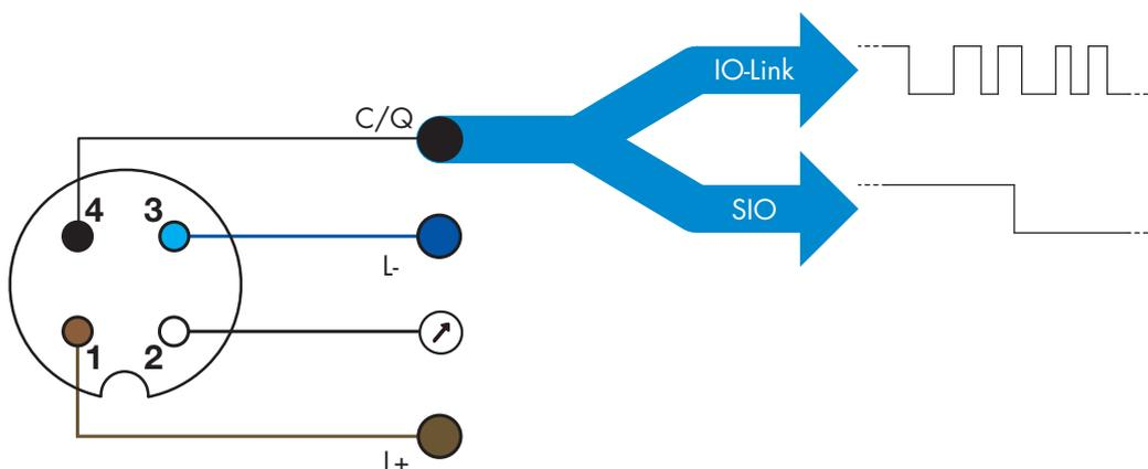
IO-Link communication takes place with a 24 V pulse modulation, standard UART protocol via the switching and communication cable (combined switching status and data channel C/Q) PIN 4 or black wire.
