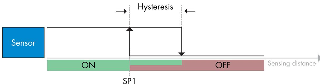
Example of presence detection - with non-inverted logic
