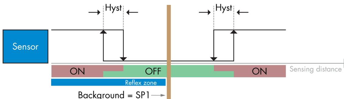
This teach-procedure affects the output of Pin4. This teach procedure saves one value for SP1 as required by the switching mode. The button is found in the Parameters menu: "Setpoint 1 Single Value Teach". Prepare the installation by mounting the sensor and preparing the background placement.
