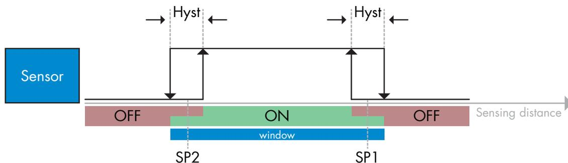
This teach procedure affects the output of Pin4. It saves one value for each of SP1 and SP2 as required by the switching mode. The buttons are found in the Parameters menu: "Setpoint 1 Single Value Teach" and 'Setpoint 2 Single Value Teach'. Prepare the installation by mounting the sensor and preparing the target placements.
