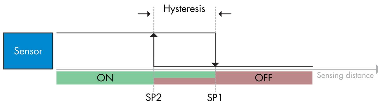
This teach procedure affects the output of Pin4. It saves one value for each of SP1 and SP2 as required by the switching mode: Two point mode. The buttons are found in the Parameters menu: "Setpoint 1 Single Value Teach" and "Setpoint 2 Single Value Teach". Prepare the installation by mounting the sensor and preparing the target placements.
