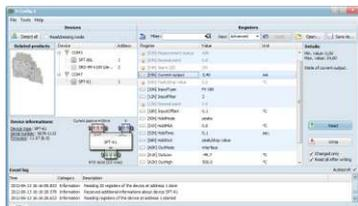
**S-Config 2** is used for the simultaneous detection of devices in multiple Modbus RTU networks and allows user to change the configuration of most of them. For each detected device a list of its registers, which the user can modify, is displayed and also additional informations about device parameters (type, address in the network, etc.).
