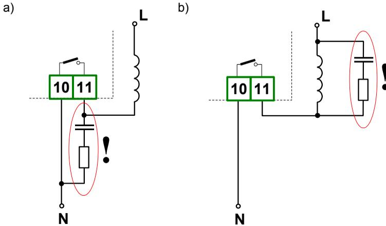
Figure 4.8. Examples of suppression circuit connection:
