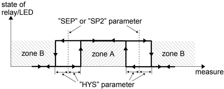
Figure 6.3. Two threshold control of the relay/LED output
