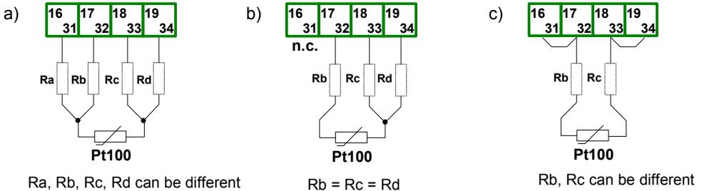
Figure 4.9. Connection of sensors:
