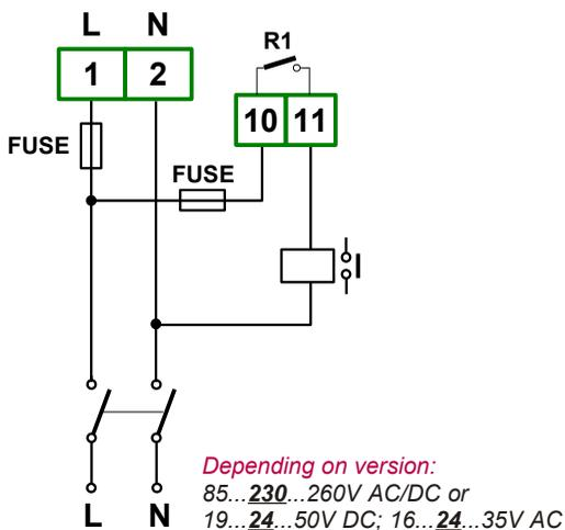
Figure 4.7. Connection of power supply and relays
