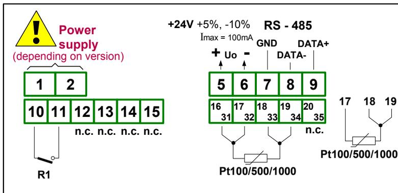
Figure 4.6. Terminals description (relay outputs, no current output version)
